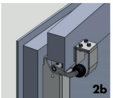
The door damper R 1400 is installed on the push side of the door. It can be attached either vertically or horizontally. There are two fixing possibilities for the hook:
