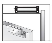
Install Z-500N bracket together with the armature plate on inswing doors.
