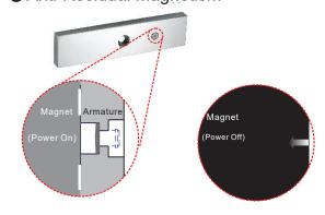
Our electromagnetic locks feature Anti-Residual Magnetism (ARM) which ensures the door can be opened without any resistance from leftover magnetism imparted to the armature plate.
