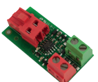
Bus Interface: Allows standard PE Beams to be used with the control board.
