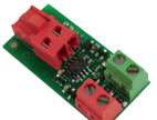
Bus Interface: Allows standard PE Beams to be used with the control board.
