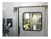
More and more machines are equipped with sound-proof enclosures to reduce the level of noise. Access to the machine usually takes place through sliding doors in the enclosure. In order for the machine to operate, the access doors must always be securely closed and a safety contact established.
